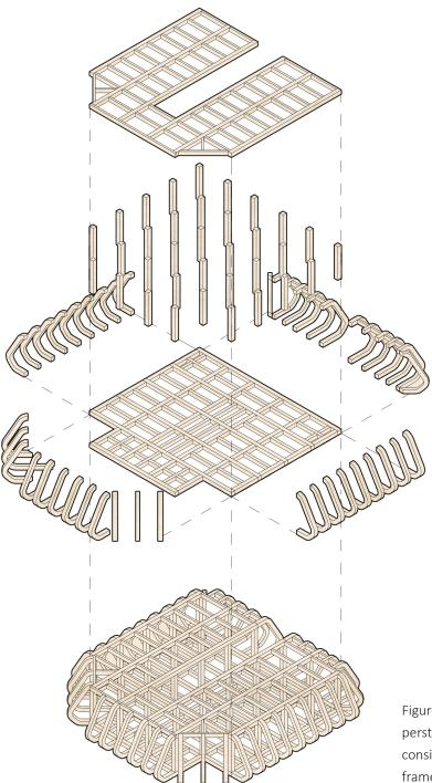
Figure 60. The structure of superstructure of the main building consists of wooden beams and frames. Original author
