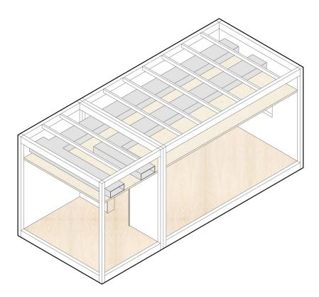
Figure 78. Prefabricated modules for main building. Original author
