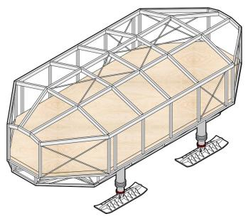
Figure 69. Module of structure construction - stage 4 steel Superstructure was installed on bottom frame. Original author
