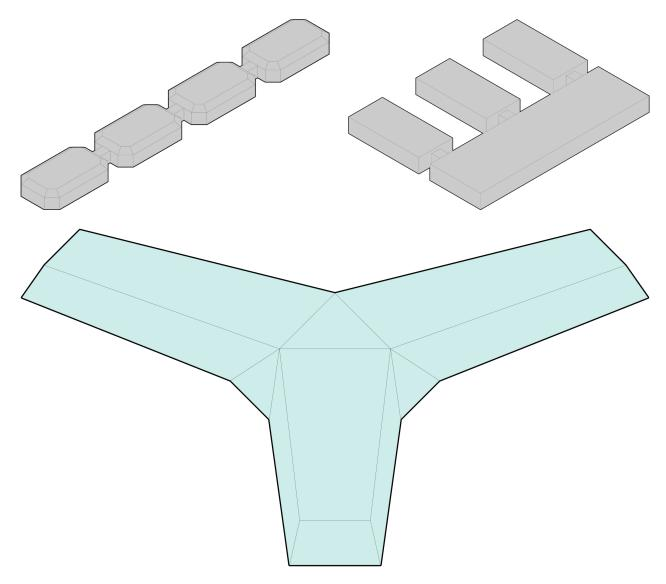
Figure 74. Linear I-type (Upper left), divided E-type (Upper right), triple arm type (Bottom). Original author. Source: Final comprehensive environmental evaluation, construction and operation of Jang Bogo Antarctic Research Station, Terra Nova Bay, Antarctica
