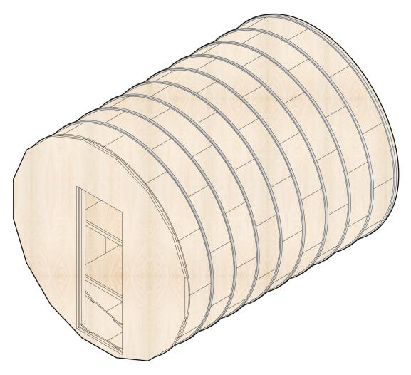
Figure 46. Construction stage 4 cover the ends of the tubes with timber frame and seal the gap of prefabricated panels. Original author
