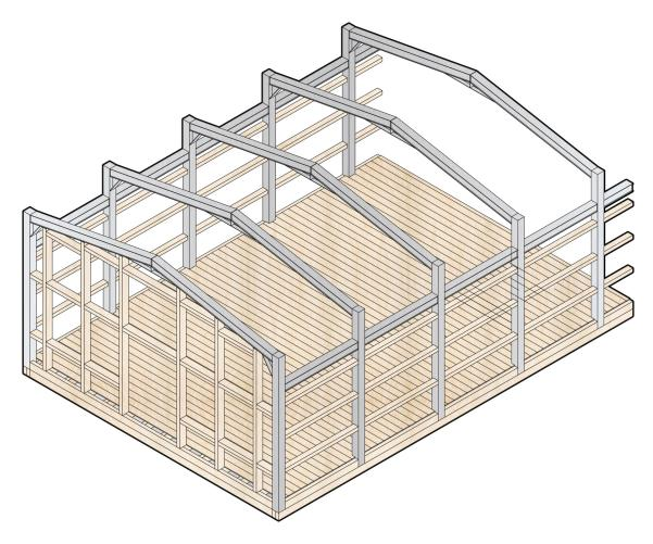
Figure 26. Construction stage 4 installing wall bracing. Original author
