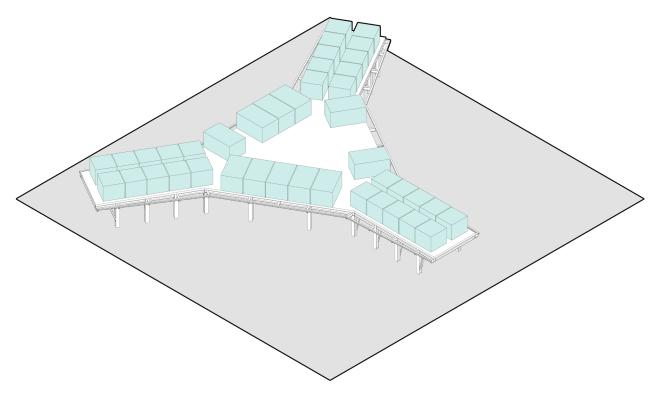
Figure 79. These modules are pre-manufactured in Korea and placed on the platform before the roof structure is installed. Original author
