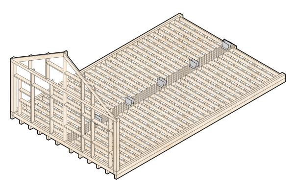
Figure 12. Construction stage 3 placing the frame of entrance to the position. Original author
