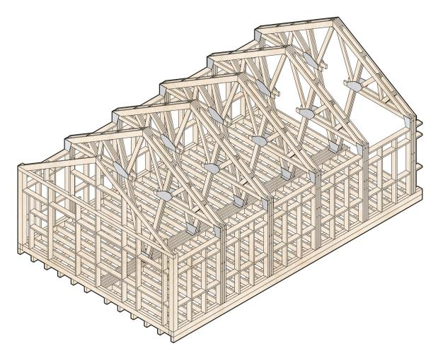
Figure 16. Construction stage 5 placing wall bracing between column to fix interior and exterior wall panel. Original author
