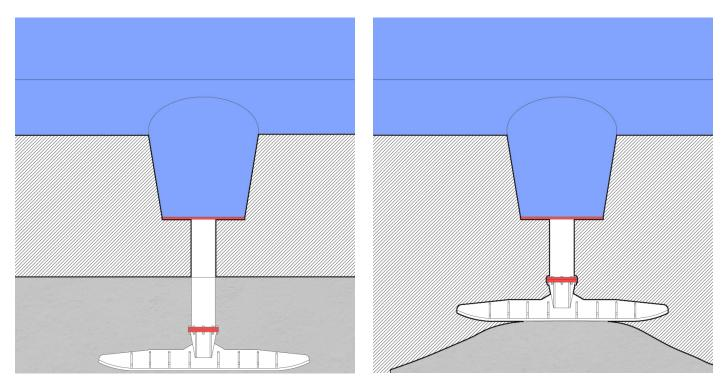
Figure 65. Hydraulically powered legs can be lifted from accumulated snow every year. Original author
