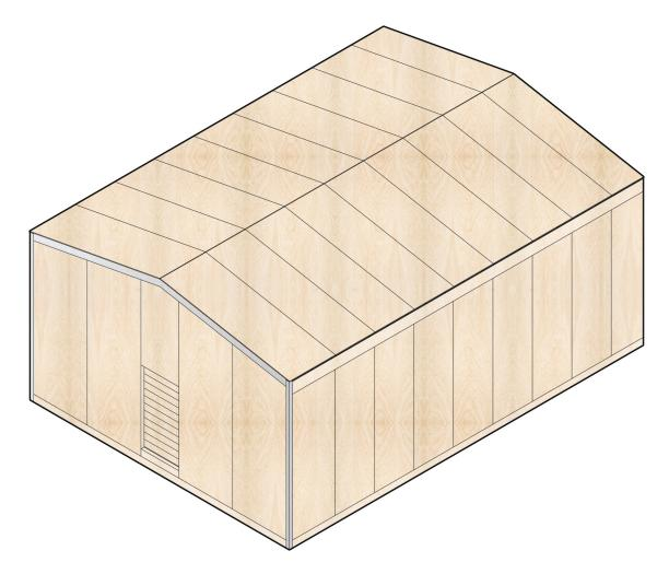
Figure 31. Construction stage 9 laid planks on the battens as the roof finish. Original author
