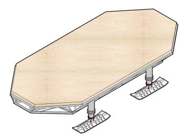
Figure 68. Module of structure construction- stage 3 Prefabricated timber floor being installed onto frame. Original author
