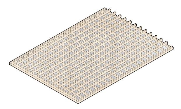
Figure 23. Construction stage 1 placing perforated metal sheet on surface and laid massive of timber on top of metal sheet to form foundation. Original author
