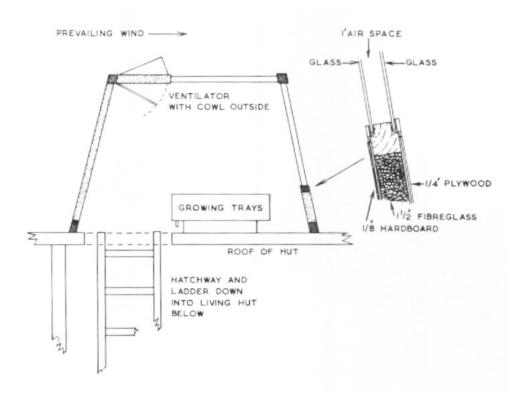
Figure 80. Construction detail of the outside greenhouse at Halley I. Photo attributed to Jack Hill. Source: https://core.ac.uk/download/pdf/31017763.pdf
