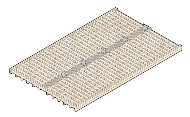
Figure 11. Construction stage 2 placing truss shoes in centre of foundation. Original author
