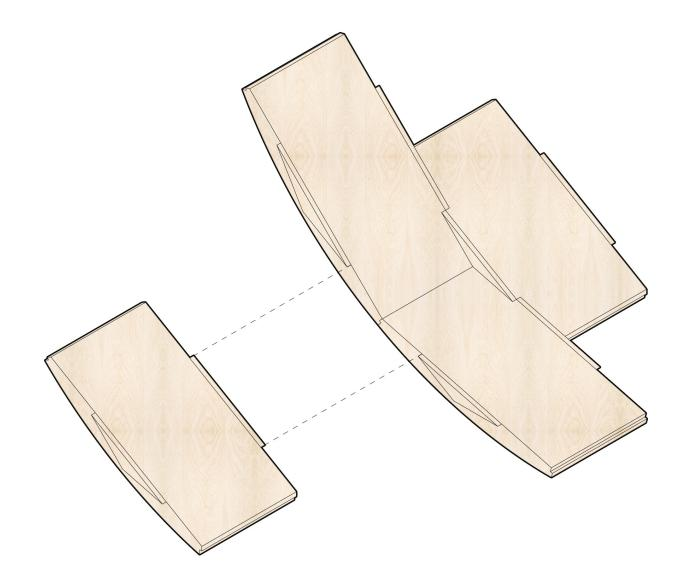
Figure 41. Each prefabricated panel can be interlocked together. Original author
