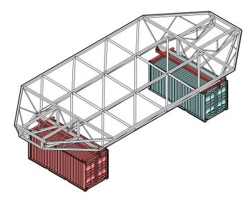
Figure 66. Module of structure construction - stage 1 The module raised on containers to allow hydraulic legs and skis to be installed. Original author
