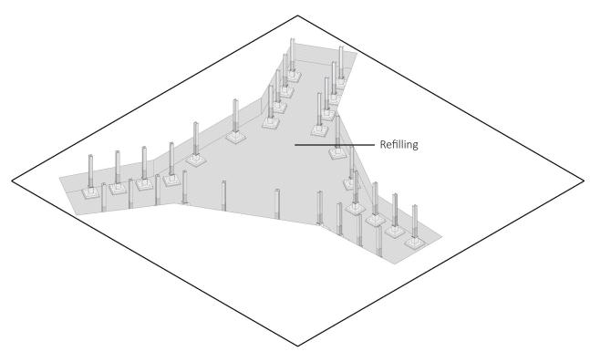
Figure 75. Foundation layout. Shallow foundation is applied to the station. Original author
