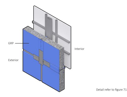
Figure 70. Exterior wall of Halley VI. Original author. Source: Ice Station the creation of Halley VI Britain's
