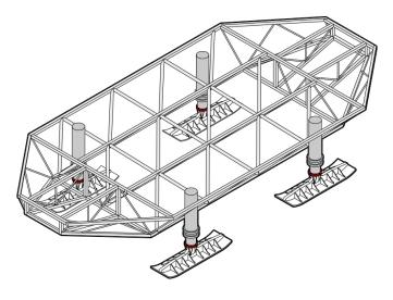
Figure 67. Module of structure construction - stage 2 Hydraulic legs and skis installed. Original author
