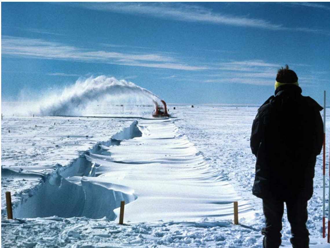
Rolba-Pete 1700k track rotary snow plough with a 2300mm wide cut in use. (A. Smith)
